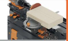
13 place wood piece onto the surface, whilst you guide the wood with the protractor for precise measurements
