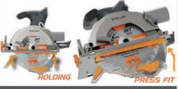
press the rear end or the Table Saw Shield support until hear it is securely held in place while holding the front end firmly.
