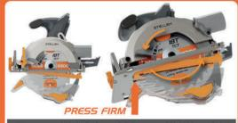
press and hold the front end of the support of the able saw shield, rotate the rear end into the rear end of the slot of the Circular Saw
