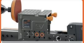
Align the holes same as seen on the diagram (orange circles) and secure the 3 screws
