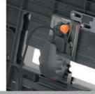
Fit the Internal Power Coupling onto the Rails on the Hotwire Cutte in where the ONE(1)GRIP connects for handheld use. Release the Slider, ensure it slides back to hold the saw in place securely.
